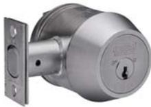
This month's product spotlight revolves around one of many deadbolts we carry. A deadbolt is a locking mechanism distinct from a spring bolt lock (lever handle) because a deadbolt **cannot** be moved to the open position except by rotating the lock cylinder. The more common spring bolt lock uses a spring to hold the bolt in place, allowing retraction by applying force to the bolt itself. A deadbolt therefore makes a door more resistant to entry without the correct key.
